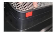
Once prime fitment is achieved, remove the condenser guard and locate the cleaning/prep pads and clean mounting surface of bumper cover. Remove the red backing from the double sided adhesive foam on all tabs. Use caution as not to touch the black adhesive surface once the red backing has been removed. Touching the black adhesive will compromise its adhering ability.
