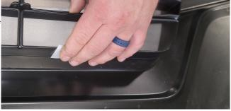
Once the condenser guard is secured in place, press firmly on all mounting tabs for 10 seconds. Inspect and adjust any tabs
