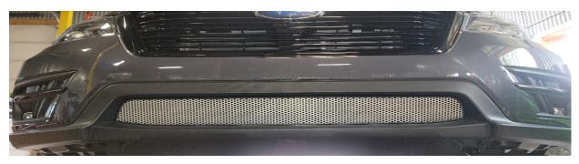
METHODS "A" & "B" both utilize an automotive grade, double sided adhesive foam for mounting. This foam also aids in protecting finishes during installation along with providing adequate adhesion properties. The adhesive foam has a red backing that should be left on during test fitting and should only be removed when you are ready to perform final installation.
