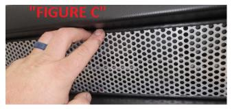
As you work from one side to the other, make sure to keep the rubber trim in front of the raised edges in "FIGURE A"
